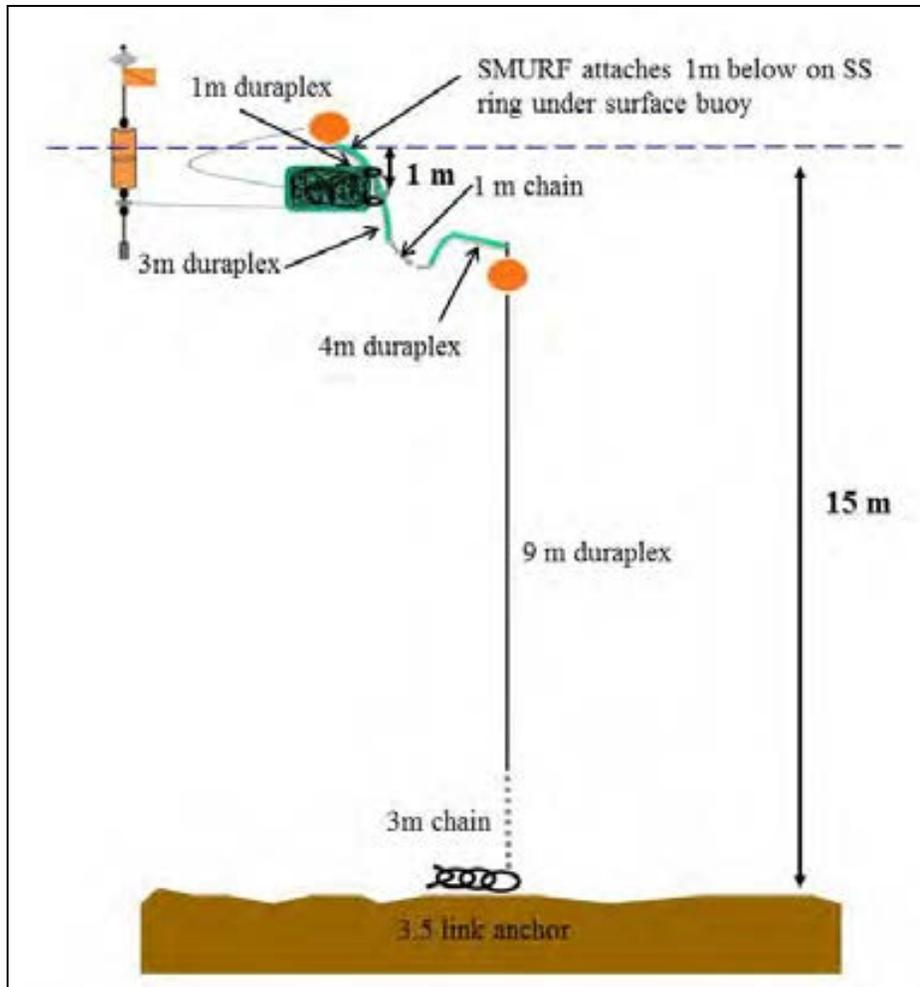
**Figure 18. Schematic of a SMURF Mooring. SMURF attached to a stainless steel (SS) ring one 1m below the surface of the water.**
